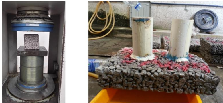
Figure 3. a) Compression Test for cube specimen, b) Infiltration Test for slab specimen
