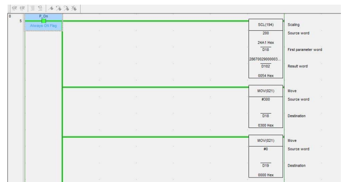
Fig. 4. Ladder diagram for flow rate calculation in manual mode
