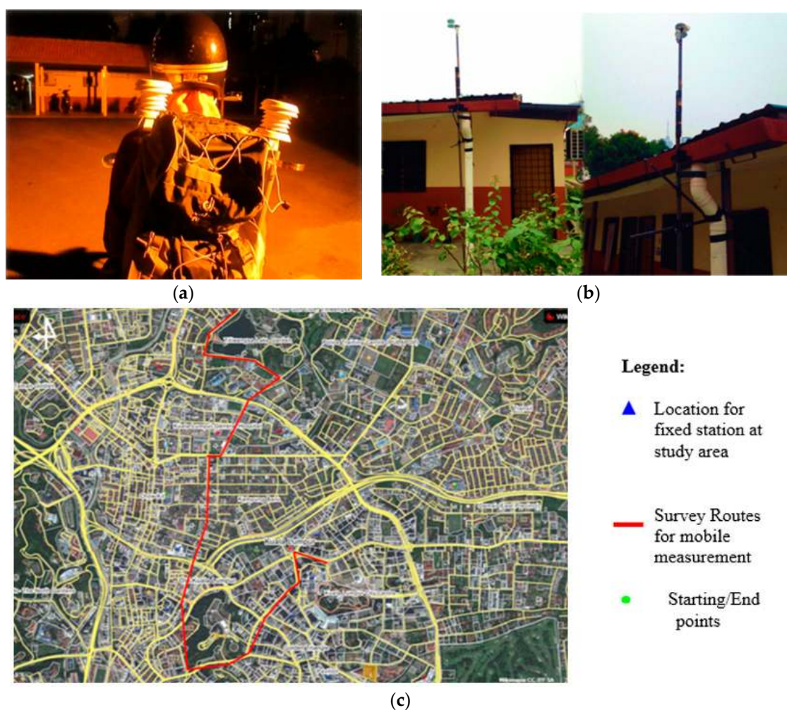
Figure 4. Mobile data collection: (a) Set-up of Hobo pro-V2 data logger with a solar radiation shield, (b) fixed station (as a control during survey) installed at SRA Raja Muda Musa, Kampung Baru. The sensors are marked in red rectangles and (c) Location of the fixed station and survey routes during the data collection at the study area.
