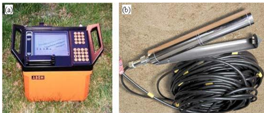
Figure 8. Seismograph and down-hole detector; (a) ABEM Terraloc MK8 seismograph, (b) downhole detector.
