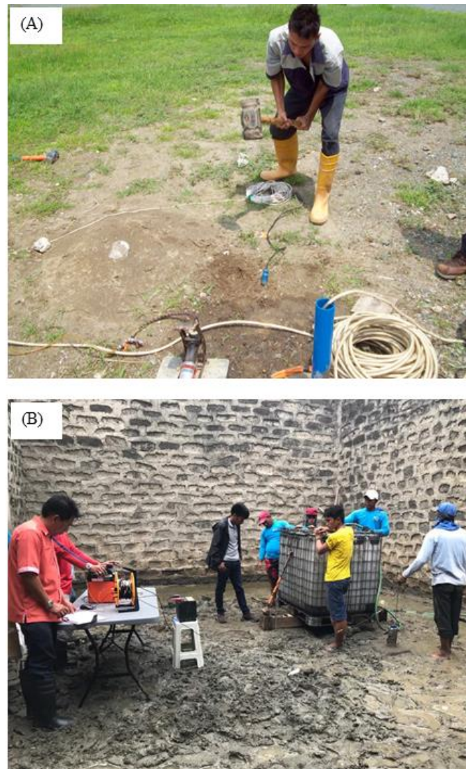
Figure 10. On-site seismic down-hole data acquisition; (A) P-wave and (B) S-waves.
