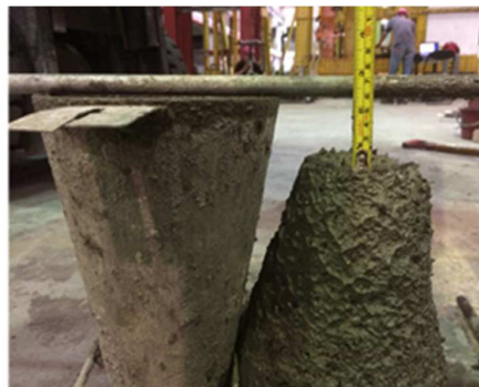
Figure 3. Fresh concrete slump
