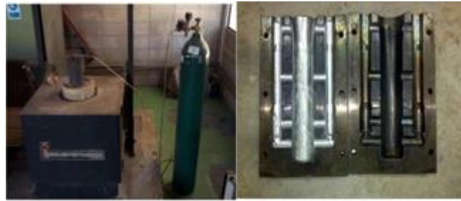
Figure 2. Induction furnace and steel mold
