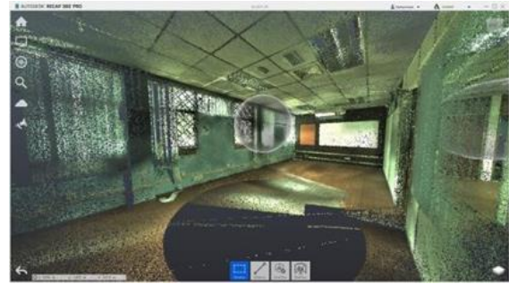
Figure 13: 3D model from TLS comes with an image.
