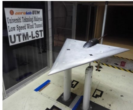
(b) Photograph of the installed VFE2 model in the wind tunnel
