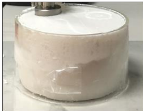
Fig. 2 - Fabricated human skin phantom
