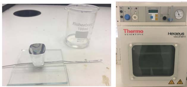
Figure 5. The RACPC-photovoltaic (PV) cell on the glass substrate and the Sylgard-184 ® solution in a beaker (left), and the Heraeus Vacutherm ™ vacuum chamber to eliminate the air bubble (right).
