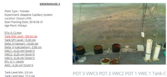
Figure 6. Dashboard for the monitoring fibrous capillary irrigation system
