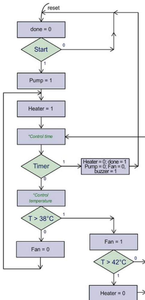
Fig. 4. The process flow of the working steps
