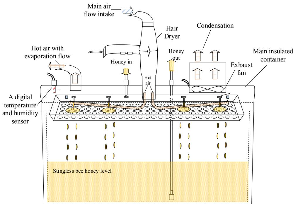
Fig. 1. The 3D Model of the Overall Prototype Design
