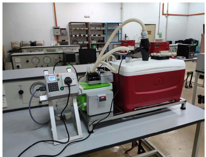
Fig. 5. The picture of the whole setup of the dehydration system
