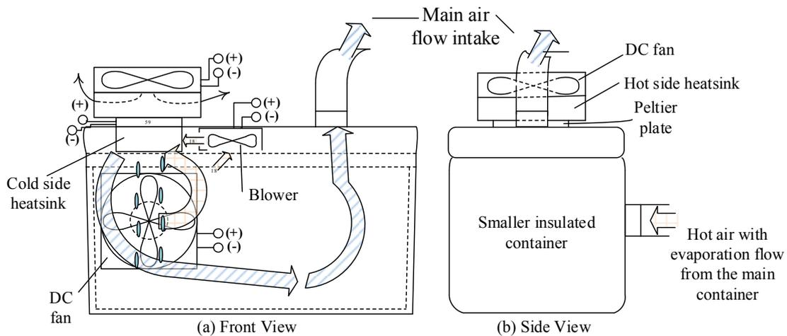
Fig. 3. (a) Front view and (b) side view of the relative relative humidity control system
