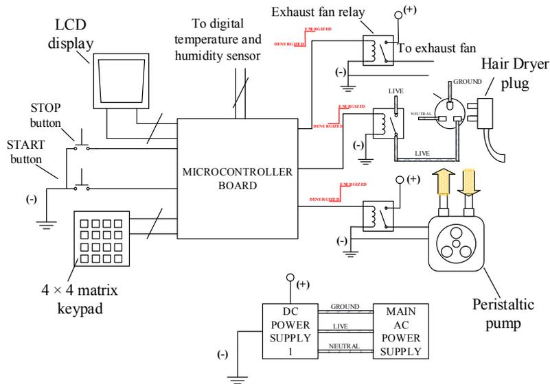
Fig. 2. Schematic of the switching/controller circuit
