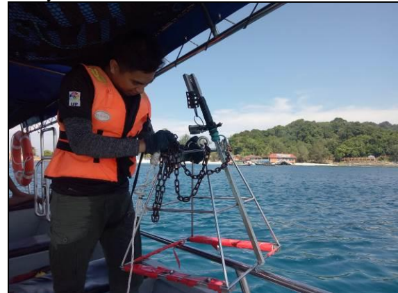
Figure 2. Visual in-situ sampling using GoPro Hero 4 mounted on a customize cage.
