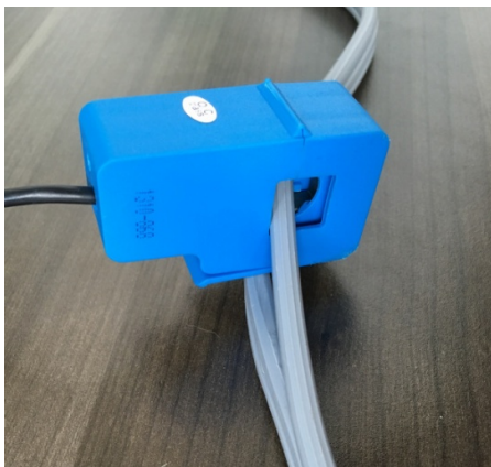
Fig. 4. Non-invasive current sensor attached to live wire
