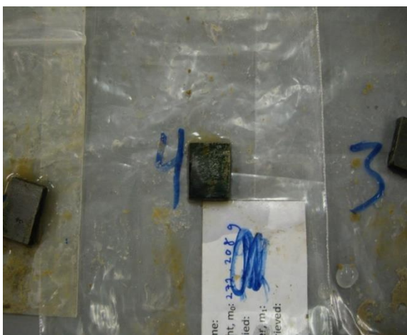
Figure 3: Coupon after retrieved from sediment
