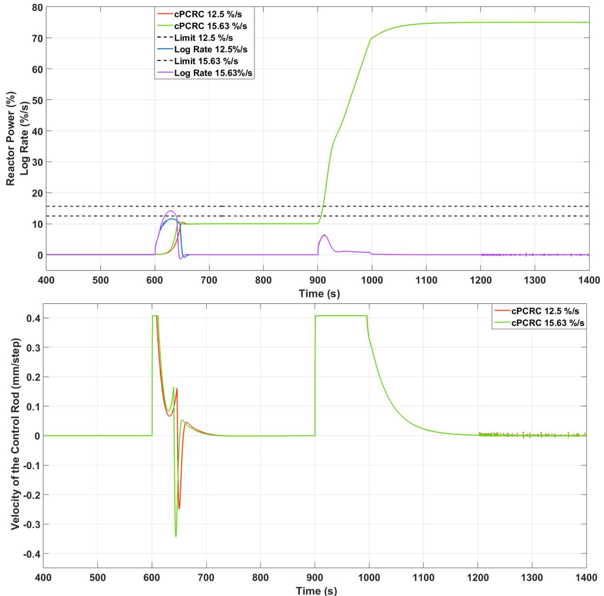
**Figure 3.** Comparison of different log rate values to limit the rate of power increment.
