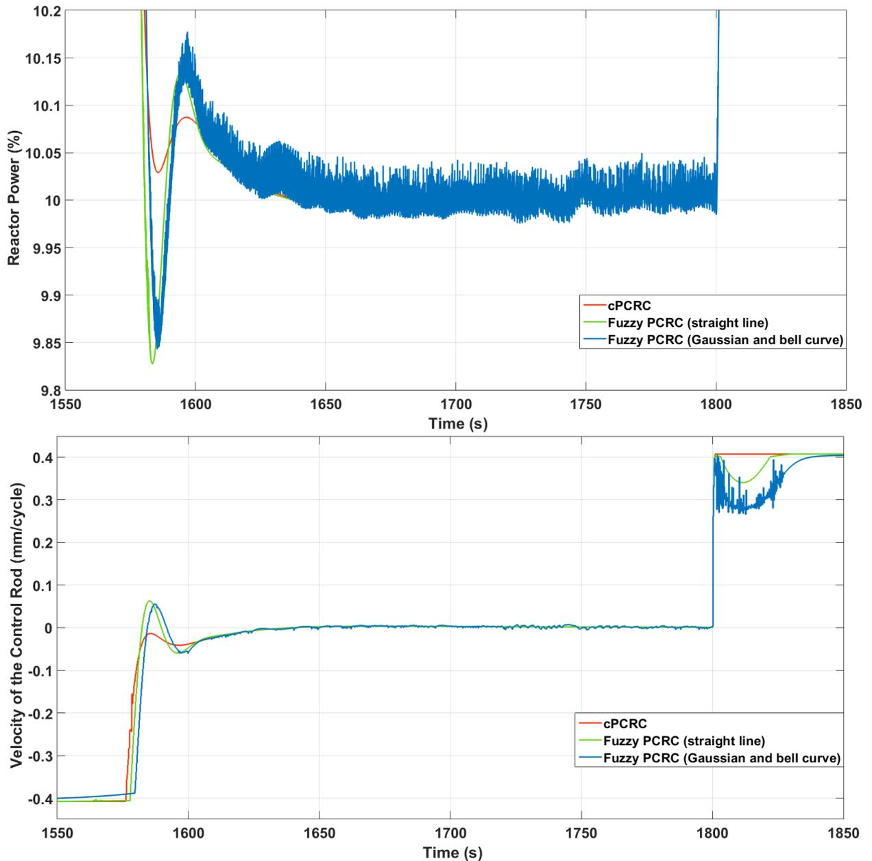
**Figure 10.** Comparison of different PCRC methods to limit the rate of power increment (by reducing the power to a lower power at 10% FP).
