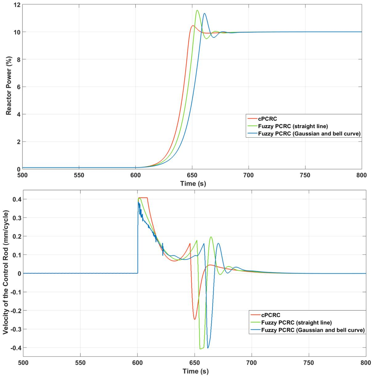
**Figure 9.** Comparison of different PCRC methods for limiting the rate of power increment (by increasing the power to 10% FP).
