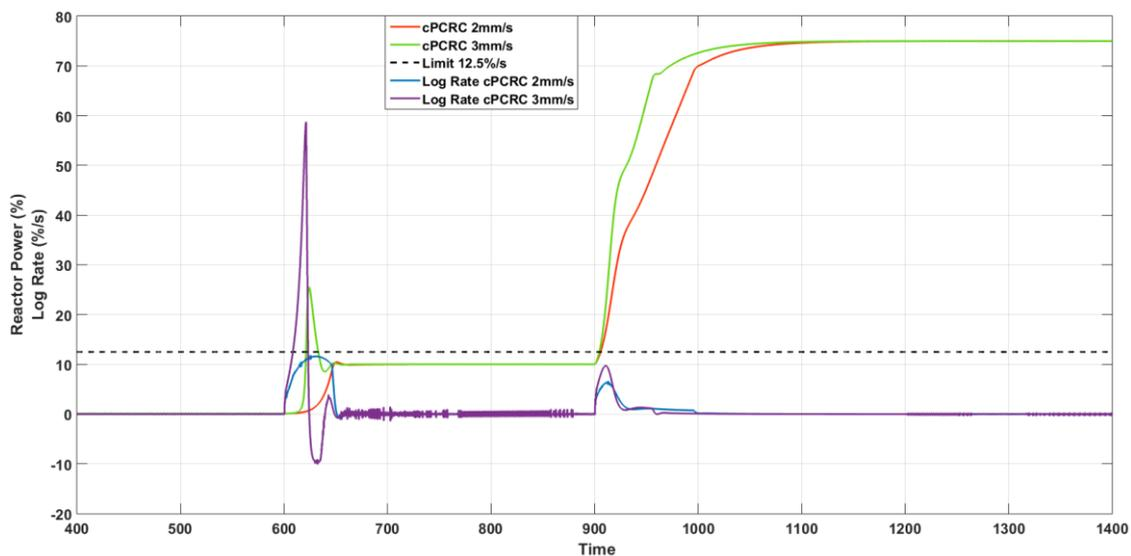
**Figure 12.** Comparison of different control rod speed values to limit the rate of power increment for conventional PCRC.
