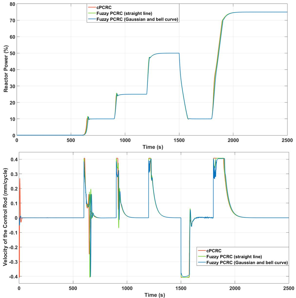
**Figure 8.** Comparison of different PCRC for limiting the rate of power increment at various steps of power change.
