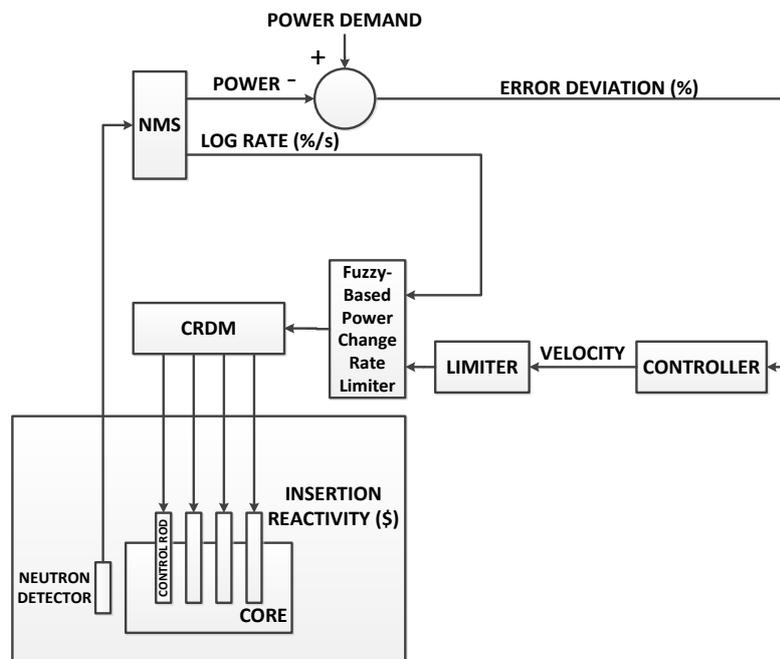
**Figure 4.** Block Diagram of Core Power Control using Fuzzy PCRC.
