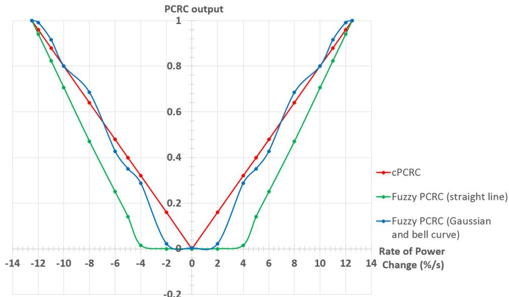
**Figure 7.** Comparison of different PCRC for limiting the input-output surface.
