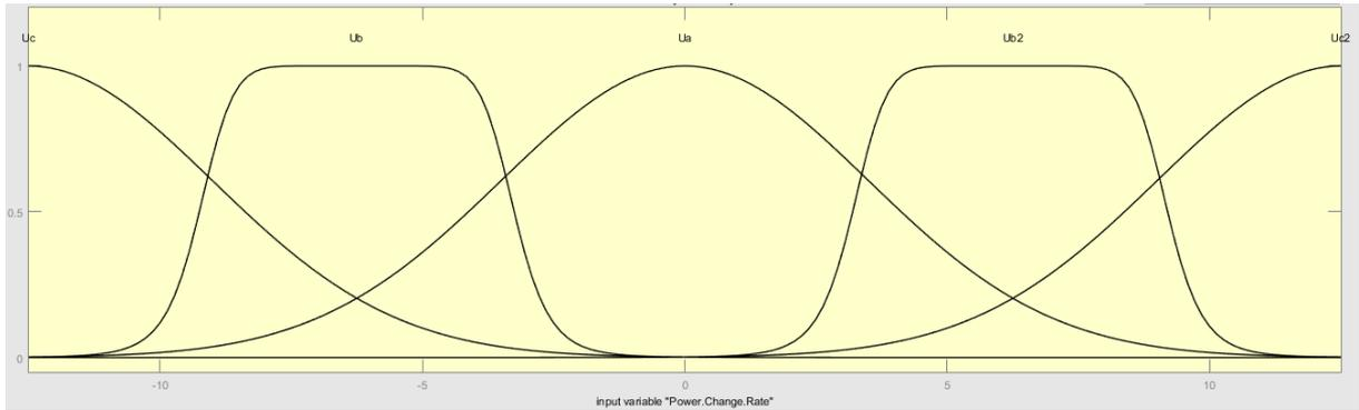
**Figure 6.** Gaussian and bell curves membership functions for Fuzzy PCRC.
