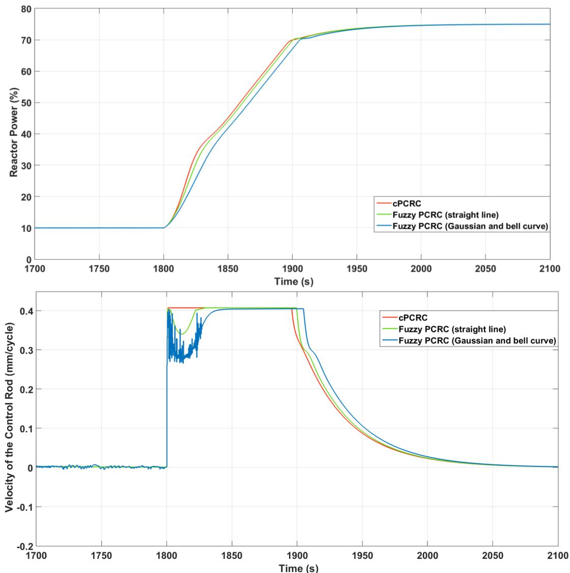
**Figure 11.** Comparison of different PCRC for limiting the rate of power increment (by increasing the power to 75% FP).
