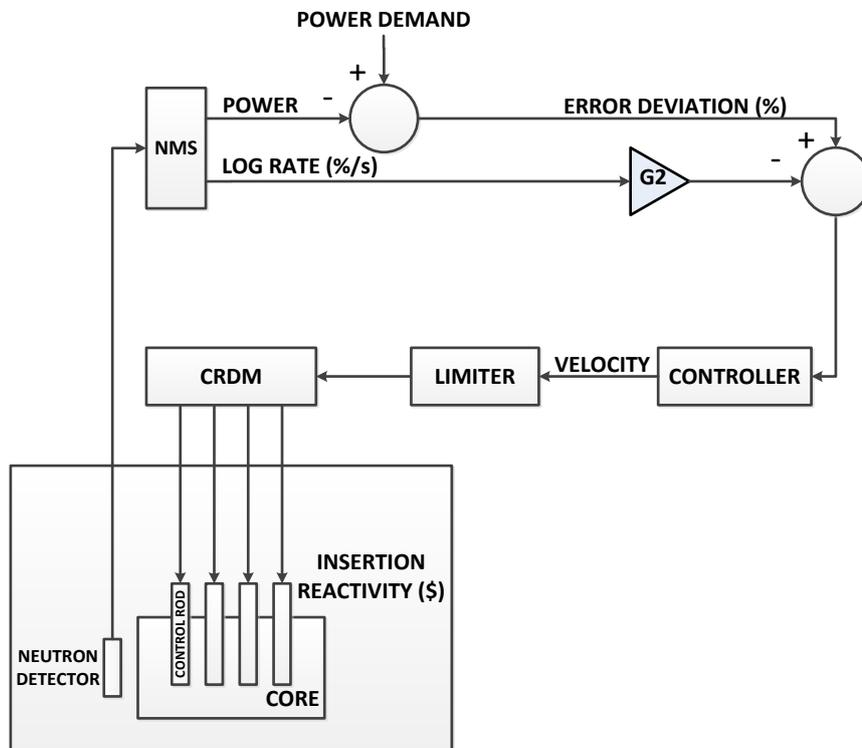
**Figure 1.** Block Diagram of Core Power Control System in RTP.
