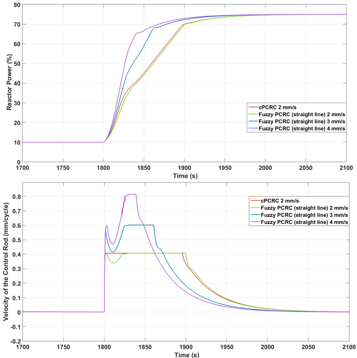
**Figure 13.** Different control rod speed values for nPCRC (by increasing the power to 75% FP).
