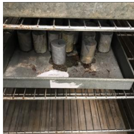
Figure 3. Drying process of limestone cored samples
