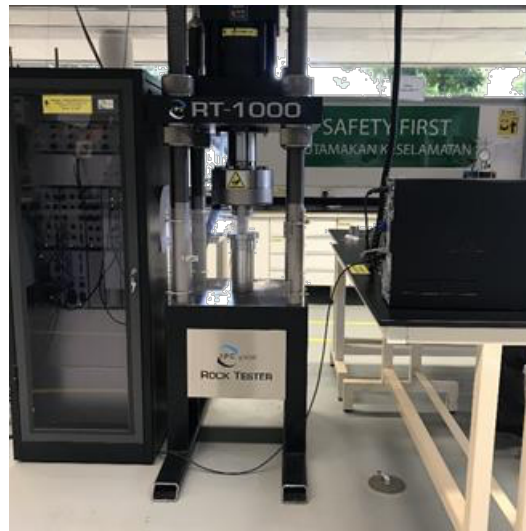
Figure 4. Uniaxial compressive test machine used for testing
