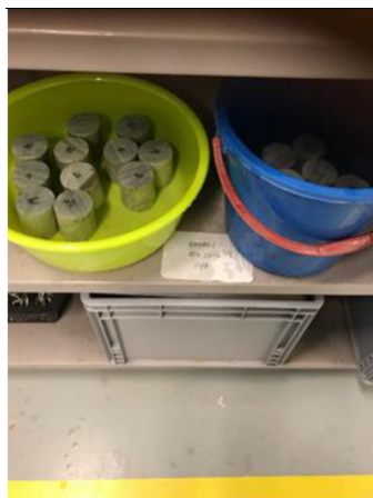
Figure 2. Wetting process of limestone cored samples
