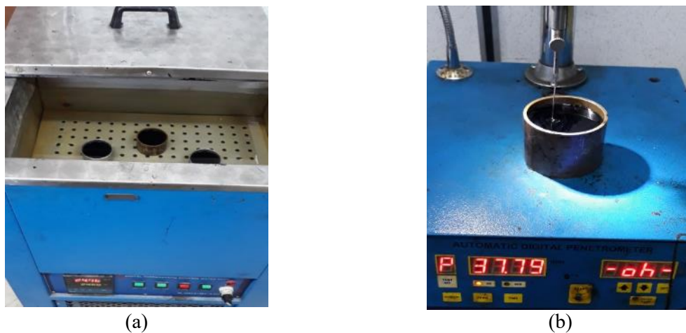
Figure 3. Penetration test set-up: (a) samples water bath conditioning (b) digital penetrometer device.
