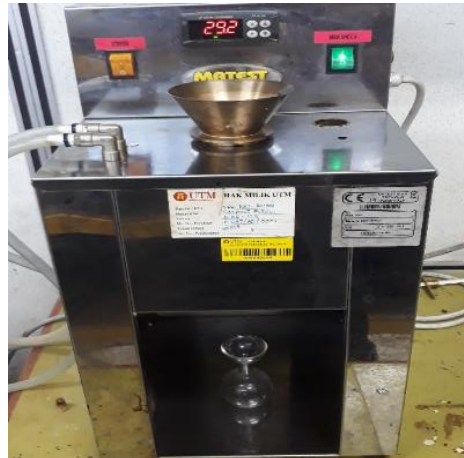
Figure 2. Experimental set-up for Say Bolt Furol Viscosity test.
