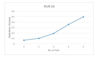
Fig. 8 - The progression wear of experiment number 10 under 90 m/min
