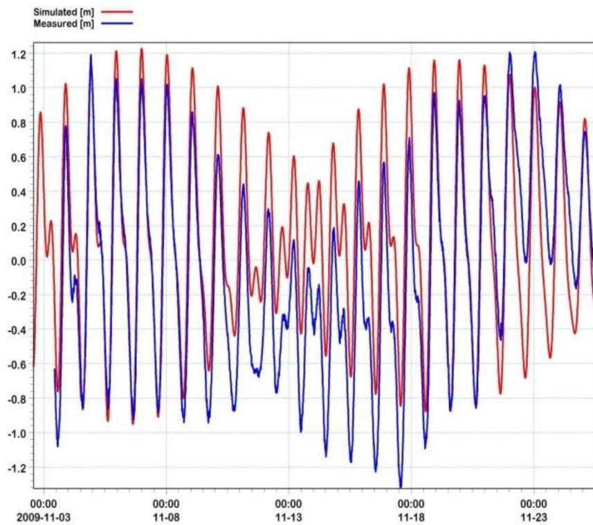
Figure 6. Calibration of water level at tide gauge
