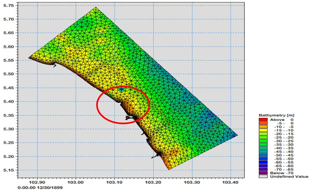
Figure 5. Bathymetry Model Domain with Triangulation mesh.
