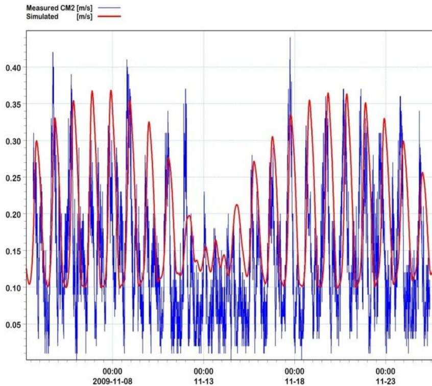
**Figure 8.** Calibration of current speed at ADCP-2.
