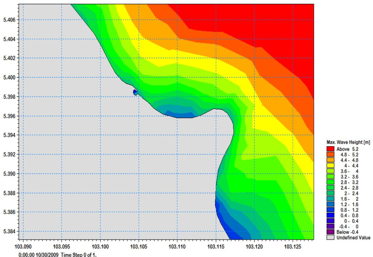
**Figure 12** Simulated spectral wave heights model result at Kuala Terengganu Airport coastal area.
