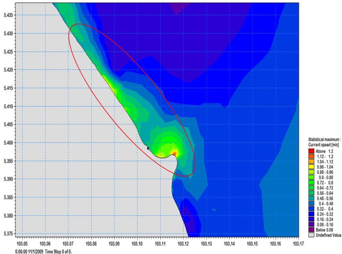
**Figure 9.** Maximum current analysis from the simulation.
