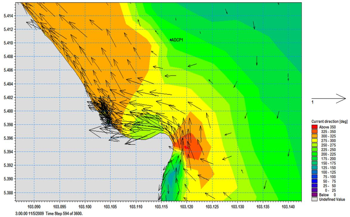
Figure 10 Current flow pattern during flood tide (Spring) at study area.
