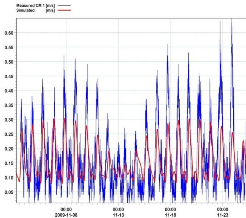
Figure 7. Calibration of current speed at ADCP-1.
