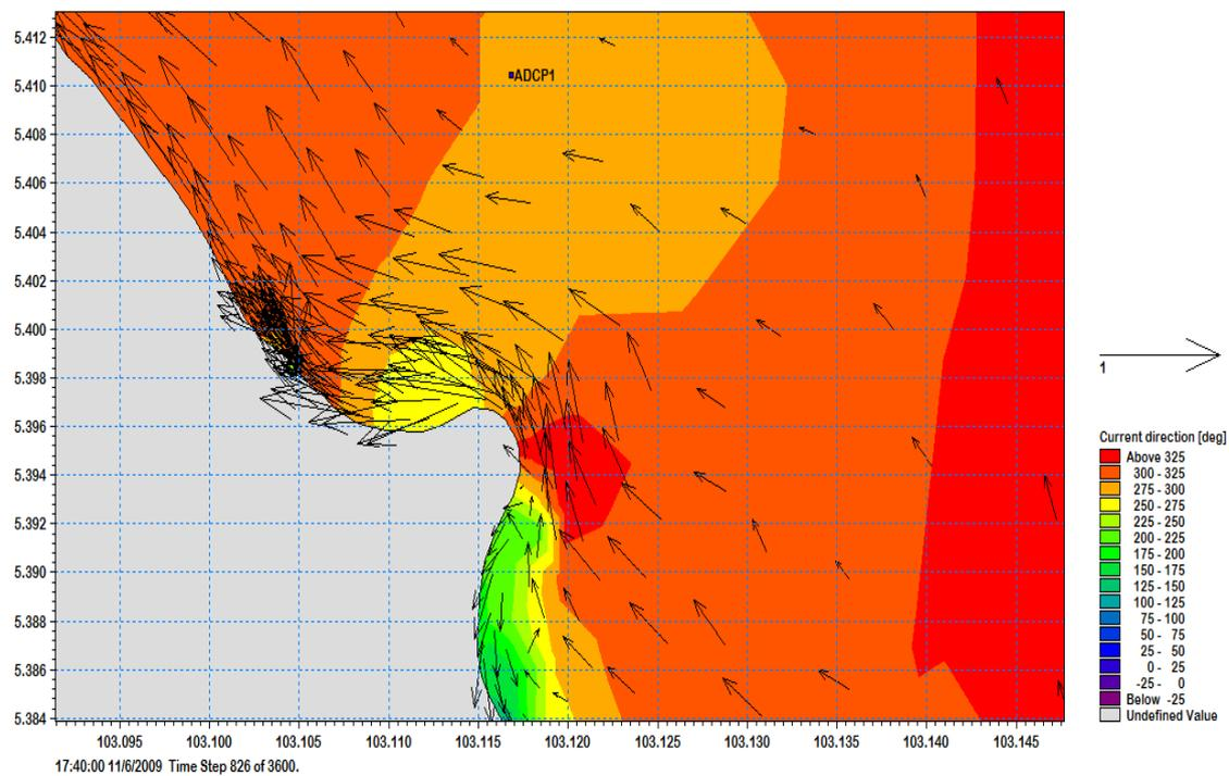
Figure 11. Current flow pattern during ebb tide (Spring) at study area.
