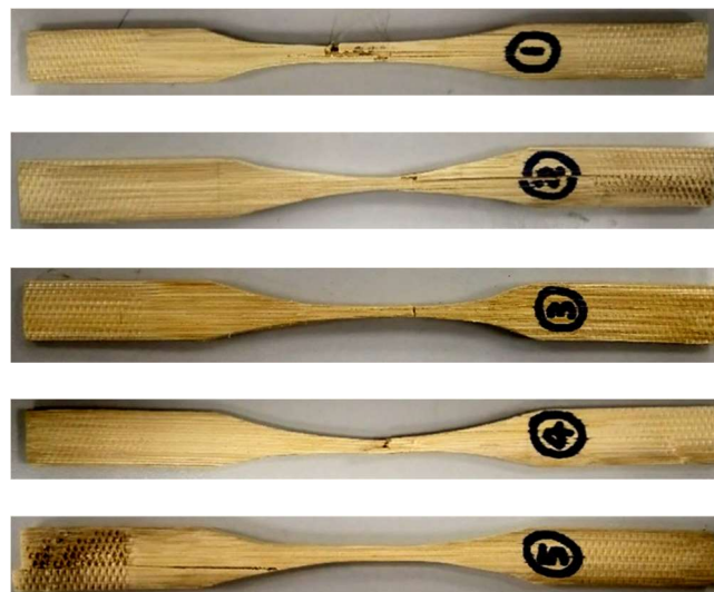
Figure 9. Failure modes of DC shape.
