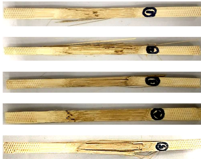
Figure 8. Failure modes of SS shape.
