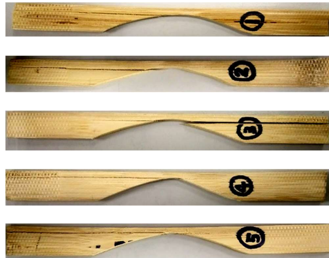
Figure 10. Failure modes of SC shape.
