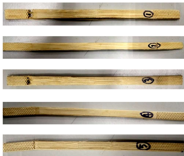
Figure 7. Failure modes of S shape.
