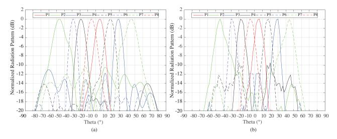
Figure 16. (a) Simulated and (b) measured main beam radiation patterns at 28 GHz for the input ports of the multibeam array antenna.
