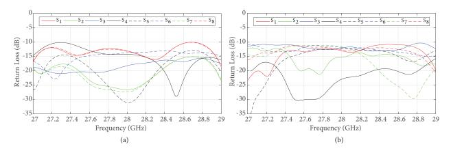
Figure 14. (a) Simulated and (b) measured return losses for the input ports of the multibeam array antenna.
