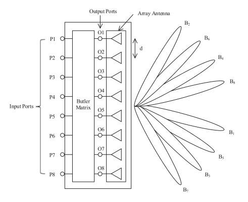
Figure 2. The configuration of a base station antenna.
