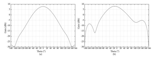
Figure 12. Simulated radiation patterns of the microstrip antenna at 28 GHz for (a) Phi=0° and (b) Phi=90°.
