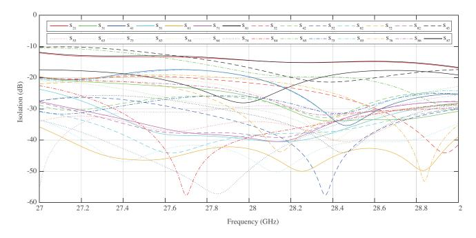
Figure 6. Simulated isolations between the input ports of the  $8 \times 8$  Butler matrix.
