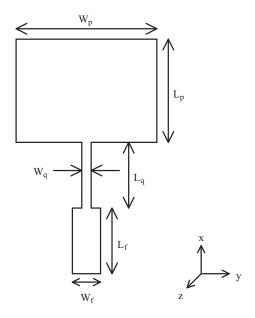
Figure 10. Geometry of a microstrip antenna.
