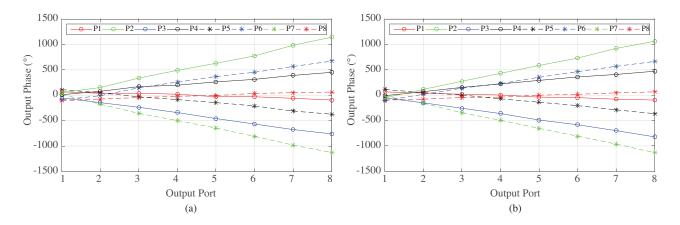
Figure 15. (a) Simulated and (b) measured output phases for the input ports of the 8×8 Butler matrix at 28 GHz.
