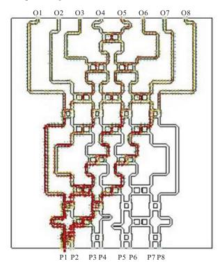
**Figure 9**. Power flow of the  $8 \times 8$  Butler matrix.
