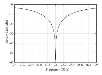
Figure 11. Simulated return loss of the microstrip antenna.
