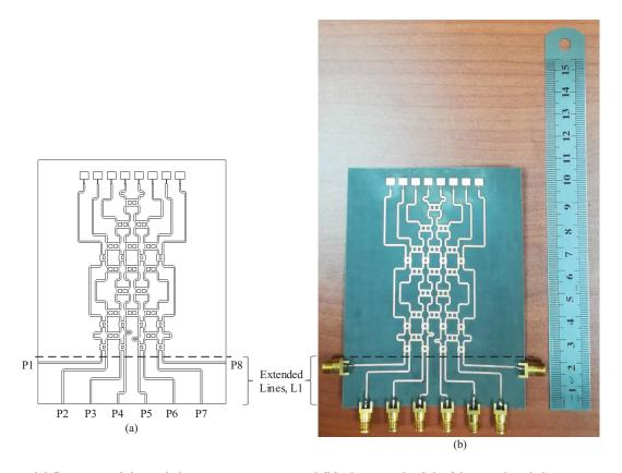
Figure 13. (a) Structure of the multibeam array antenna and (b) photograph of the fabricated multibeam array antenna.
