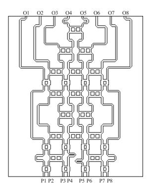
**Figure 4**. Designed structure of the  $8 \times 8$  Butler matrix.
