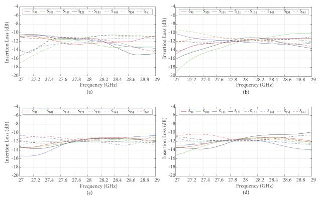
Figure 7. Simulated insertion losses of the 8×8 Butler matrix for ports (a) P1, (b) P2, (c) P3, and (d) P4.
