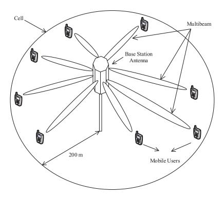
Figure 1. A multibeam base station.
