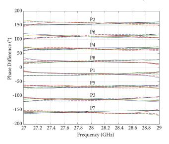
**Figure 8**. Simulated phase differences for the input ports of the  $8 \times 8$  Butler matrix.
