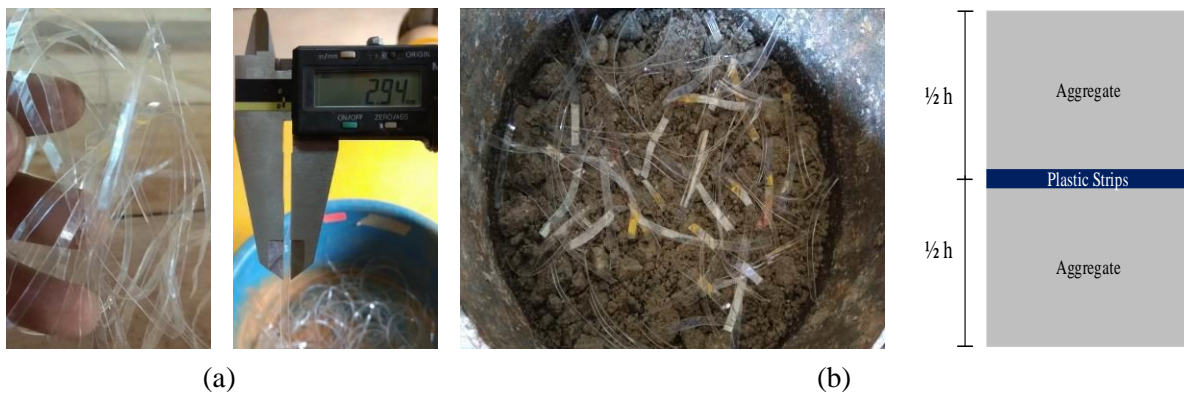
Figure 11. (a) Plastic strip from plastic bottle and (b) Plastic strip from plastic bottle and its placement.
