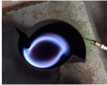
Fig. 1. Typical vortex flame in an AVC
