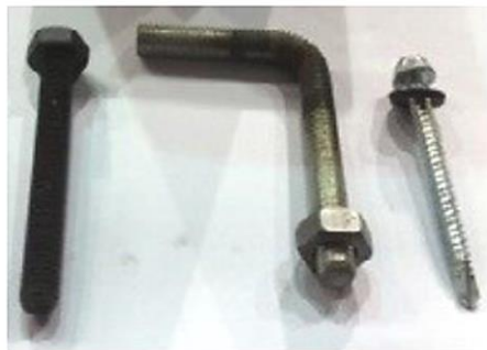
Figure 7. Proposed shear connectors; Saggaff et al., [23]
