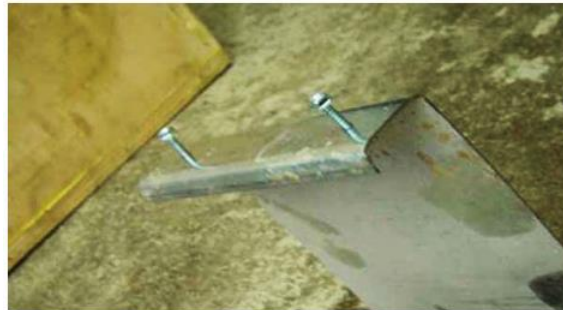
(c) Self-drilling screws installed on CFS flange
