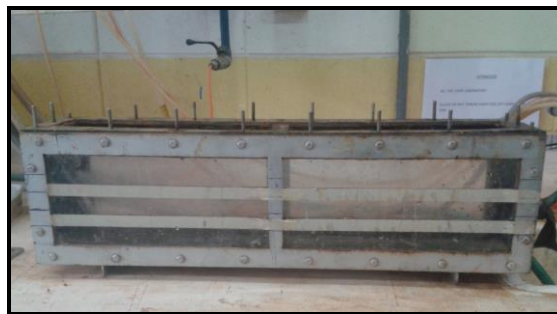
Fig. 2- Modified constant head permeability equipment
