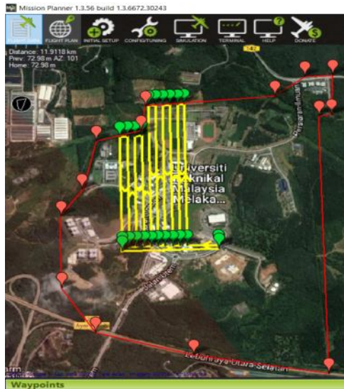
Figure 8: Waypoints of the third flight plan covering 53.93 Hectare of the study area
