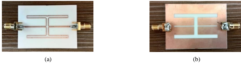
Fig. 6 -The prototype of 5G parallel coupled line band pass filter with PGS implementation: (a) front patch; (b) ground patch
