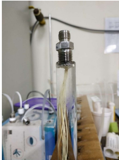
Figure 5. PDMS 3% wt (in n -hexane) coated P84 co-polyimide membrane.
