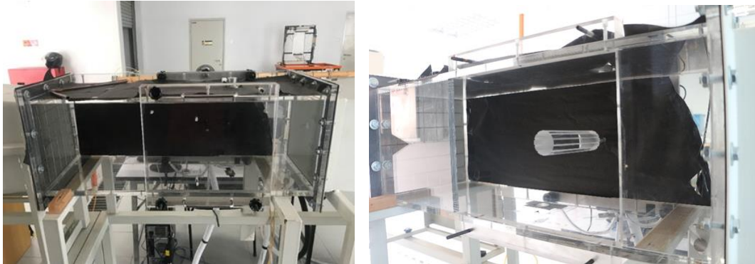
Fig. 4. Cylinder test model installed in the test section
