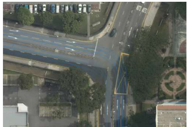
Figure 2. Blue lines indicate the outlines of multiple overlapping scan tracks for a single road.
