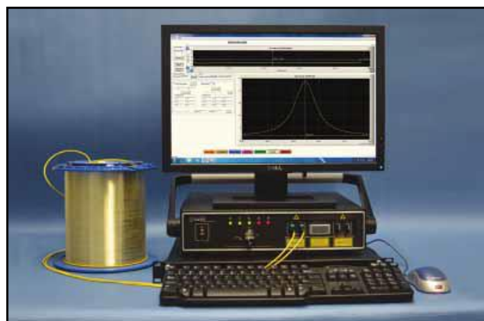
Figure 2. Fiber Optic Distributed Strain and Temperature Sensors (DSTS) BOTDA Interrogator. ( www.ozoptics.com )
