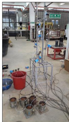
Figure 4. Calibration of tensiometer acquisition system.
