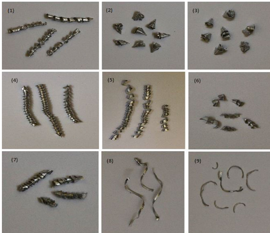
Fig. 7 Chips collected for each experiment on A5083
