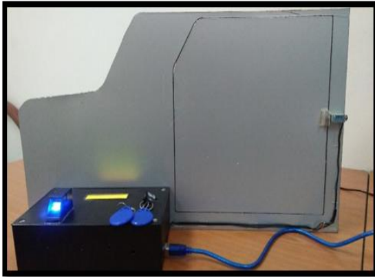
Fig. 6. Prototype of Vehicle Door Security using Smart Tag and Fingerprint System
