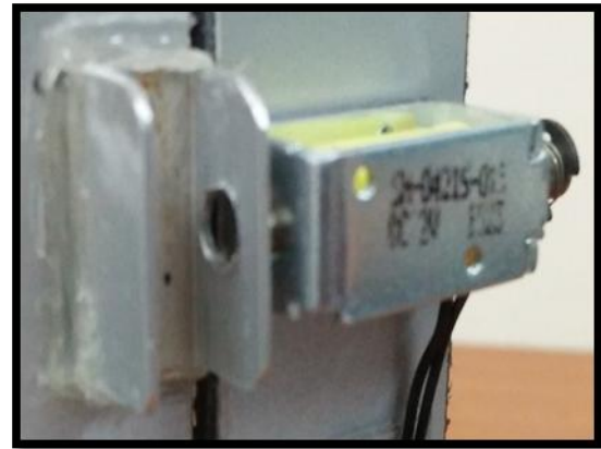
Fig. 9. The motor will function to lock and unlock the door
