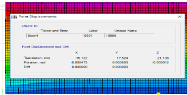
Fig.8. displacement at roof level-south part of the building in Etabs T.D.P models for period 70 years
