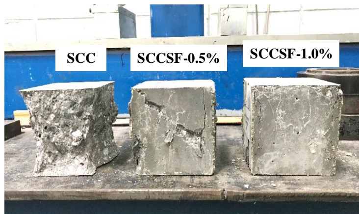
Figure 6. Comparison of Cube Test Failure Mode for SCC, SCCSF-0.5% and SCCSF-1.0%.
