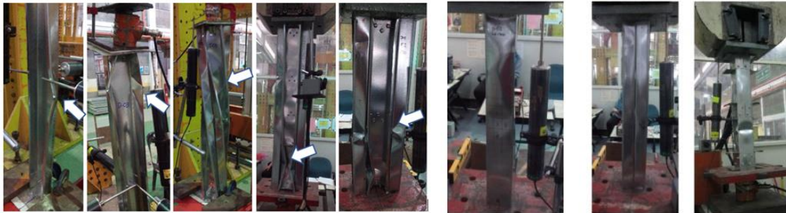
Figure 2. Basic performance cold-formed steel when received axial load
