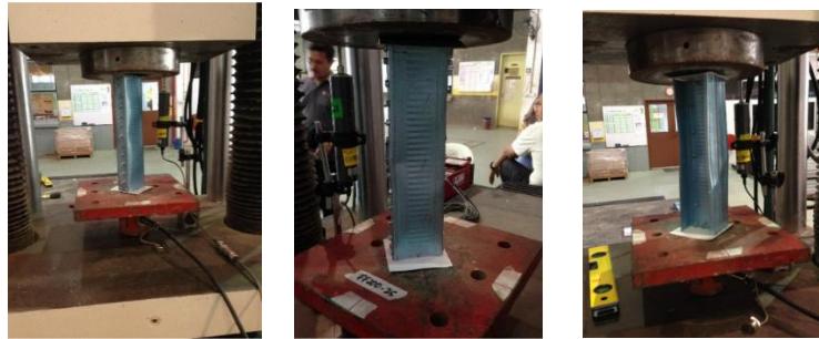
Figure 6. Compression test machine Tunius Olsen.
