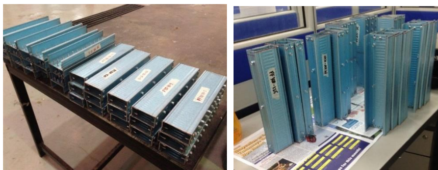
Figure 4. Samples with variable screw distances.
