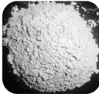
**Figure 2.** Ground granulated blast furnace slag (GGBFS) sample [8]
