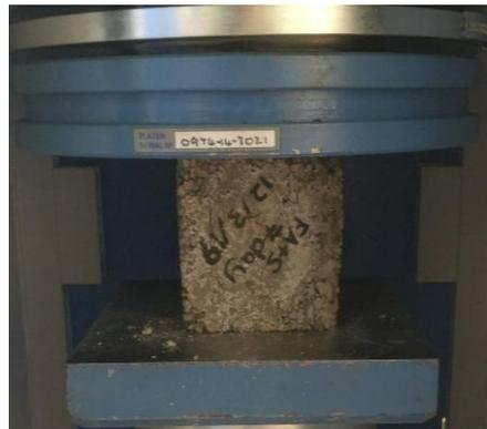
**Figure 3:** Compressive strength test
