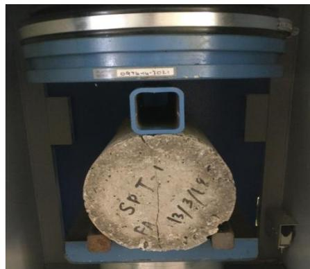
**Figure 4:** Splitting tensile strength test
