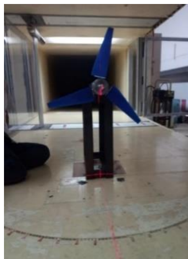
Fig. 15: The wind turbine model is fixed in the testing section of UTM LST wind tunnel.
