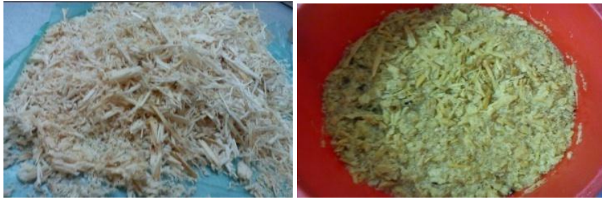
Figure 1. Bagasse fibre image: (a) Bagasse fibres drying process under sunlight, (b) Bagasse fibre soaking process in 1% NaOH solution.
