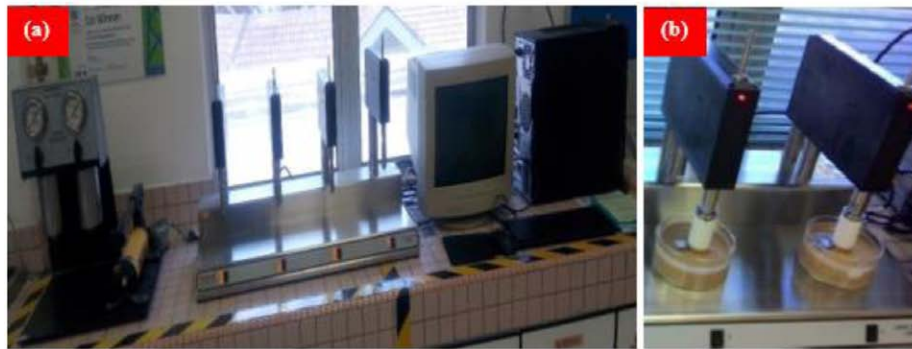
Figure 3—Experimental (a) set up; (b) test of SASO and diesel mud samples with LSM
