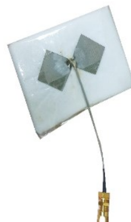
Fig. 6. Prototype of textile diamond dipole antenna [3].
