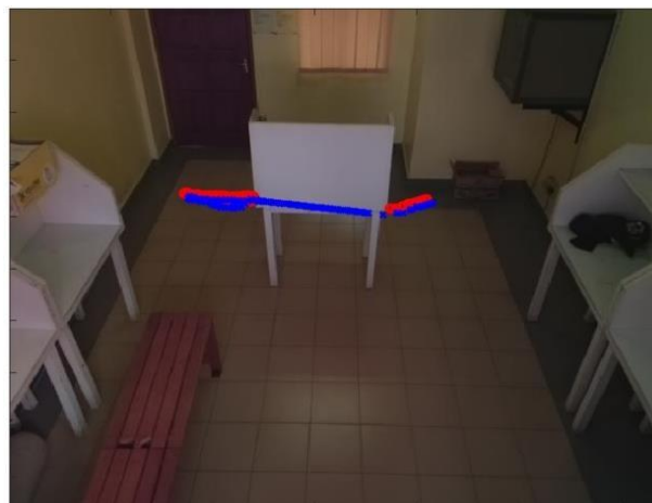
Fig. 15 - Decoy's detection results using template matching (red dots) and Kalman filter (blue dots)
