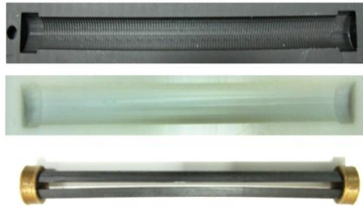
Figure 3. Actuator mold. From above – Inner mold, outer mold and rod with holder
