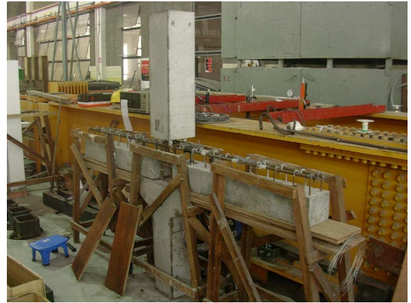
(b) Precast specimens ready for wet connection
