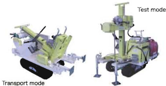
Fig. 3. Transport and test mode of Screw Driving Sounding equipment [9].
