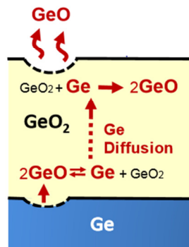
Fig. 5. Desorption mechanism of thermally oxidized Ge surface.
