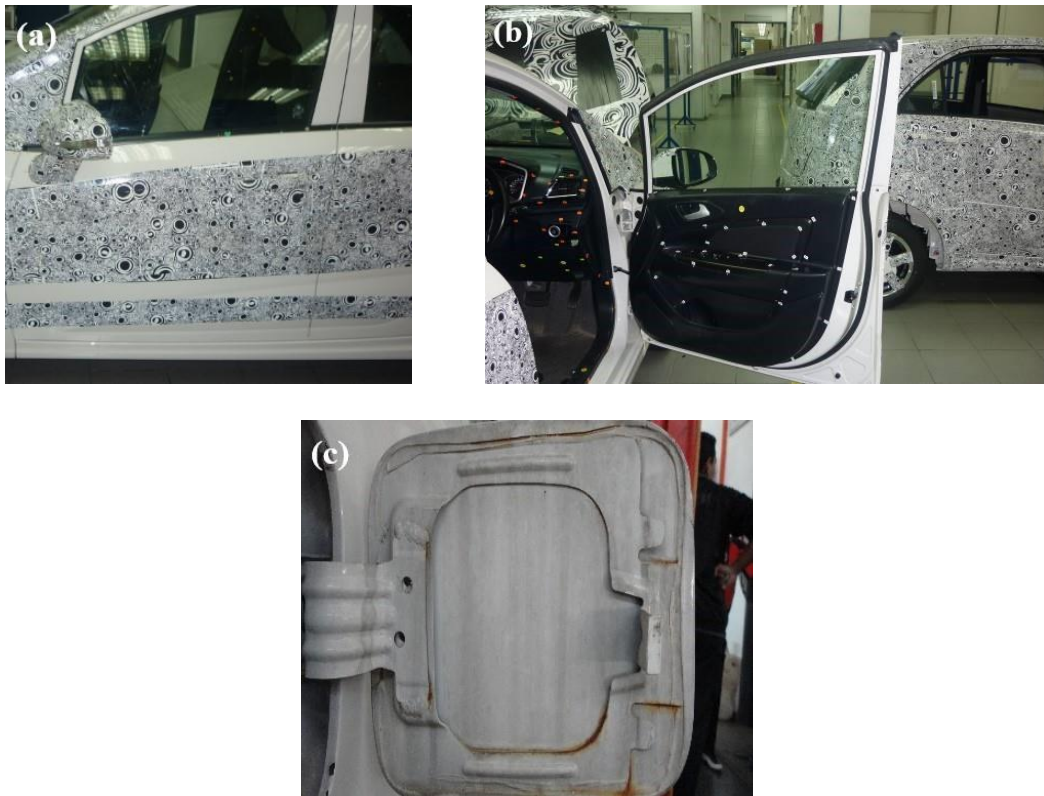
Figure 6. (a) exterior of vehicle, (b) secondary surfaces at door panel and; (c) bleed of rust at fuel filler lid.
