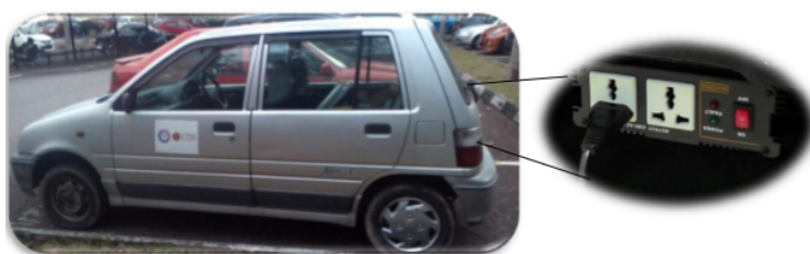
Fig. 1. Physics on the Go (PotGo) in Mobile Computer-based Physics Laboratory (MCPL) with DC-AC converter
