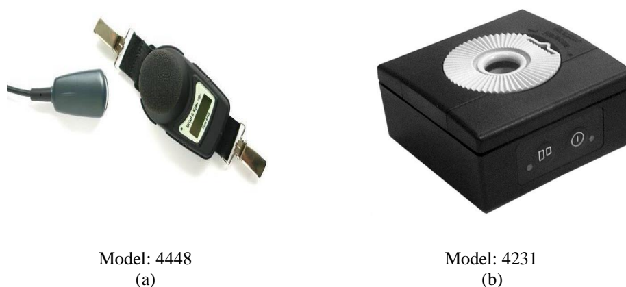
Figure 2 (a) Noise dosimeter and (b) calibrator for personal noise monitoring
