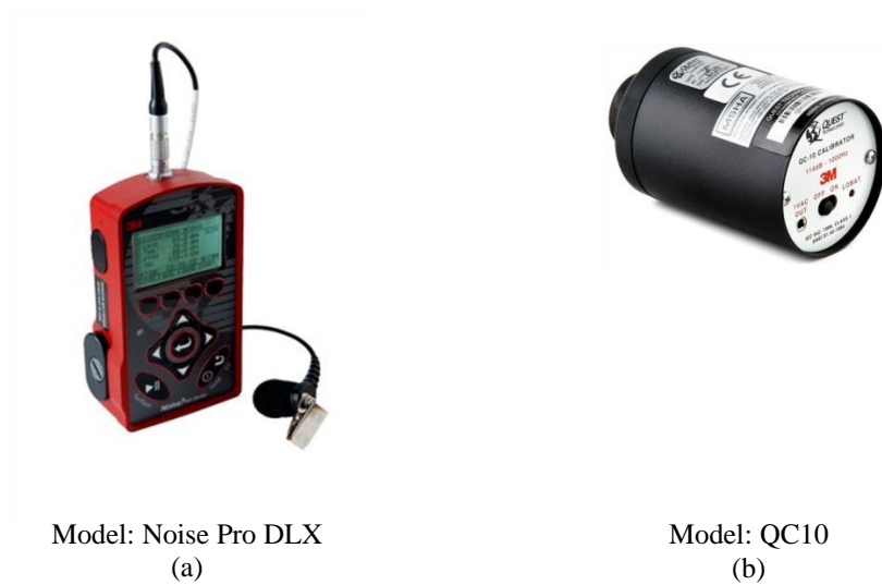
Figure 1. (a) Noise dosimeter and (b) calibrator for noise monitoring at working area
